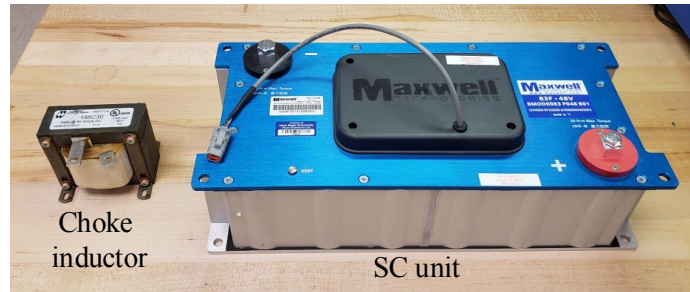
Fig. 4.53: Elements of the energy buffering unit: Maxwell BMOD0083 P048 B01 SC module and a choke inductor.
