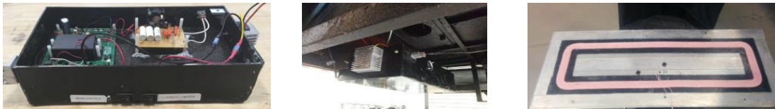
Fig. 3.17: Transmitter circuit hardware, and TC structure.
