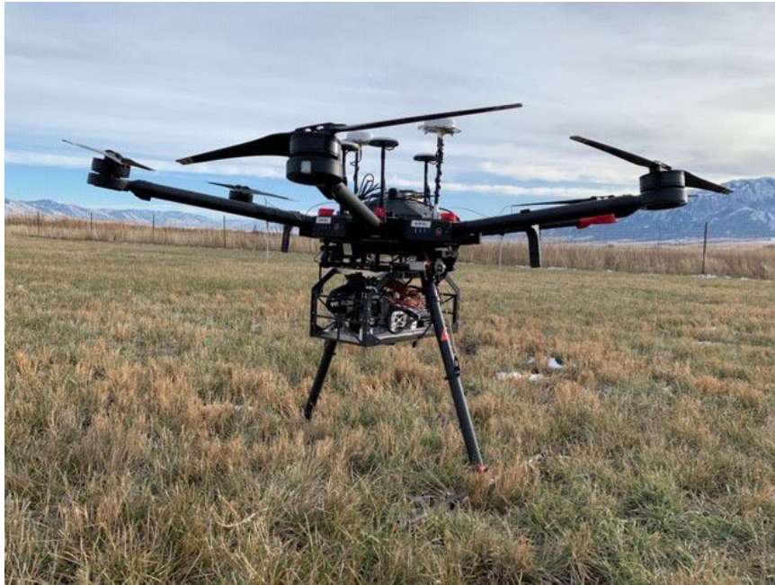
Fig. 3.5: Texel camera mounted in the DJI rotorcraft.
