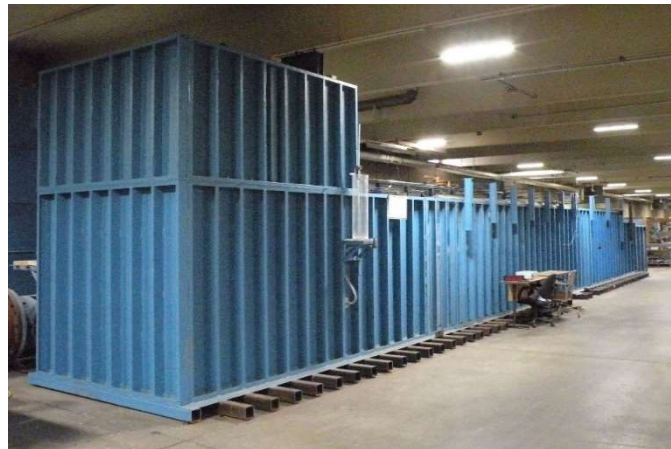
Fig. 2. Photograph of the flume in the UWRL.
