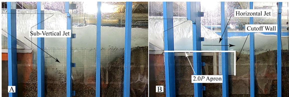
Fig. 25A and B. Run 14 (A) in comparison to Run 23 (B) for the fine substrate, Q = 300 l/s, and h_d = 0.17 m (Table 4). Run 23 has significantly less scour due to L_a = 2.0P .
