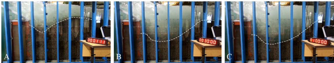
Fig. 15A-C. Scour development with time for (A) Initial Phase, (B) Second Phase, and (C) Final Phase (timer displays time of observation).
