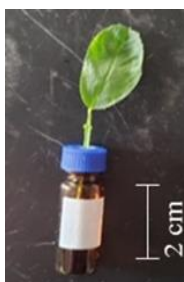
Figure 8. Alfalfa Leaf Setup for Photodegradation Experiments. For real experiments the stem of the leaf was threaded through the cap further so that the leaf was in a more stable position.
