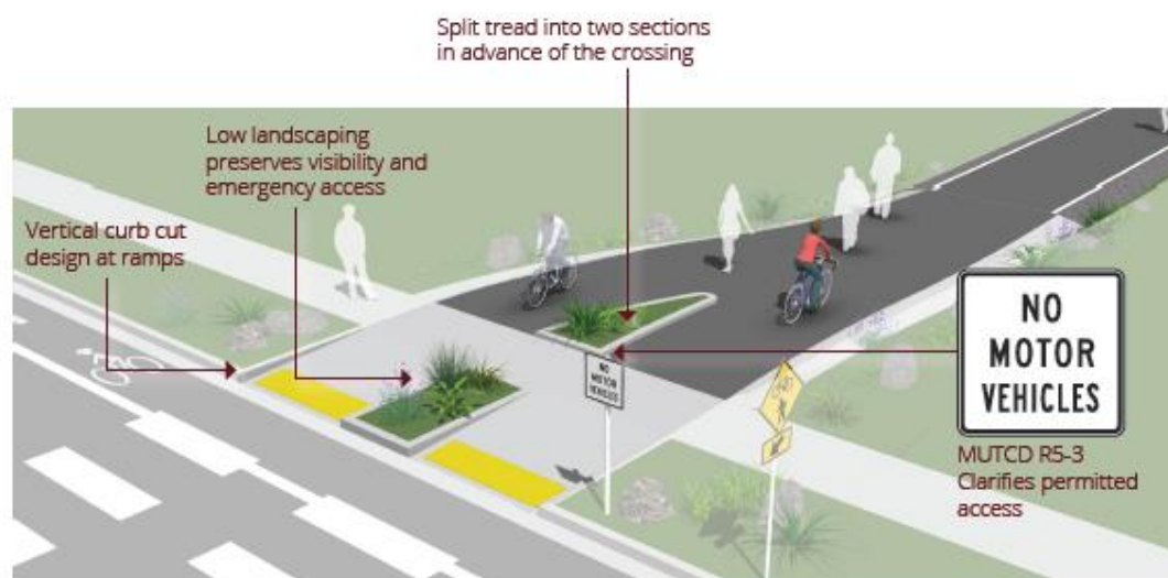
Figure 4-12. Access control treatment method (Alta Planning + Design).
