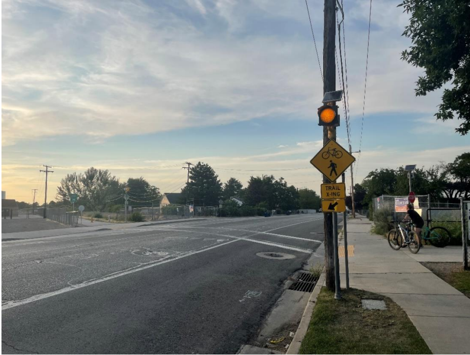
Figure 4-9. Pedestrian activated crossing light at canal trail intersection.
