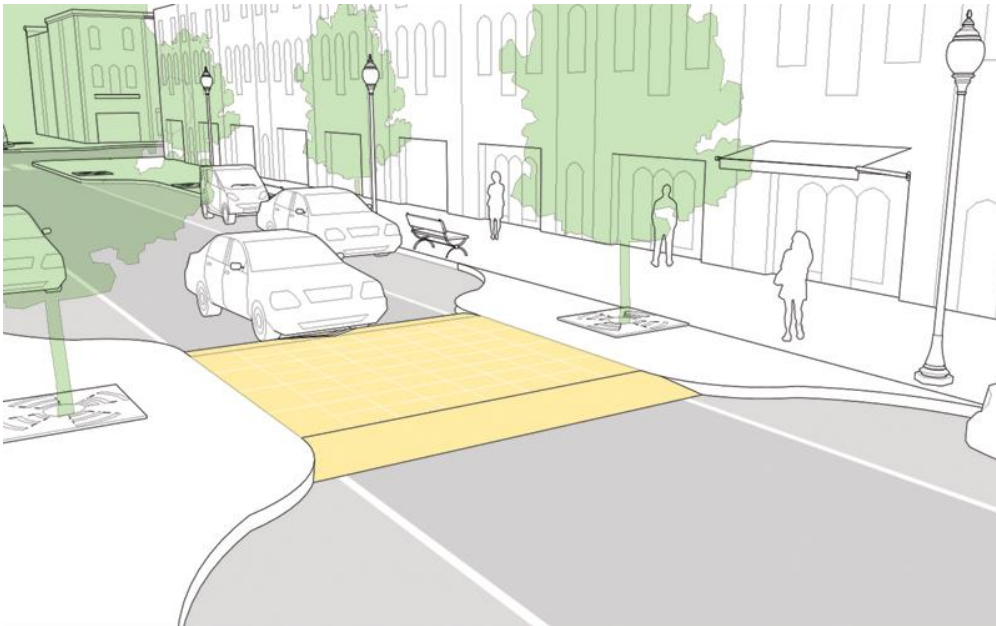
Figure 4-1. Speed table crossing treatment used at trail access points (NACTO, 2012).
