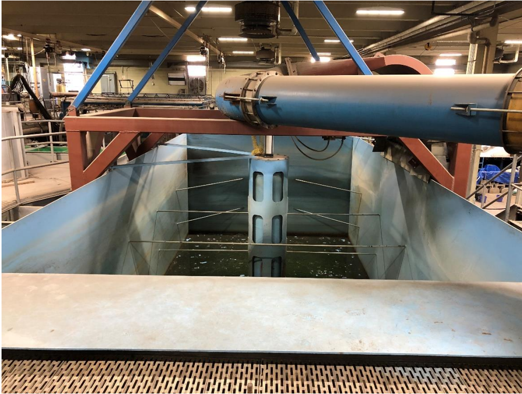
Figure 13. 250,000 pound NIST traceable weight tank
