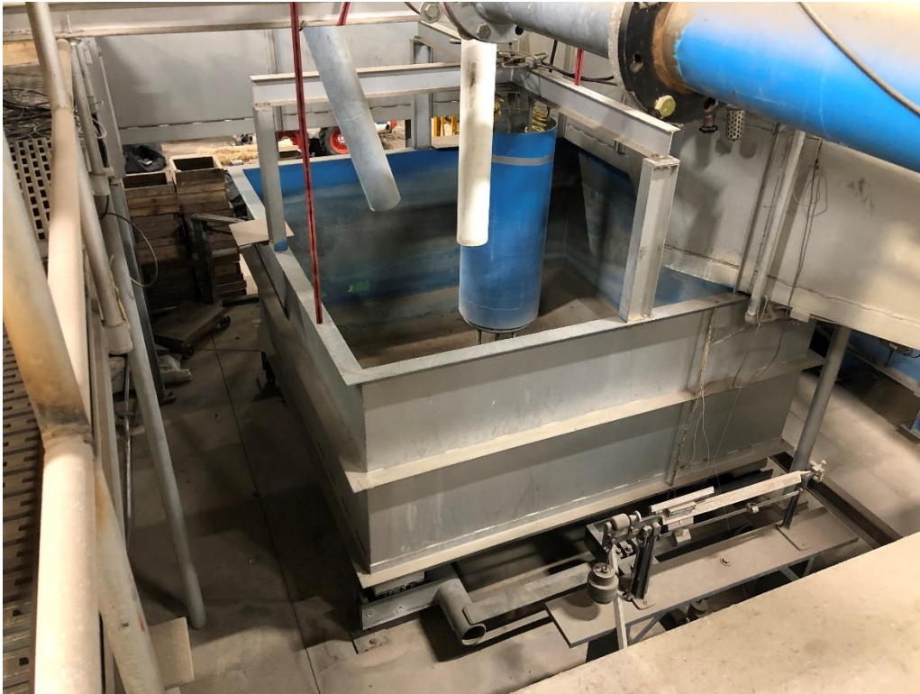
Figure 12. 25,000 pound NIST traceable weight tank
