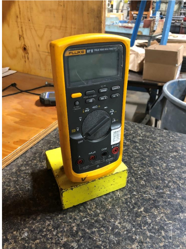
Figure 9. Multimeter used to average total flow and differential pressure.
