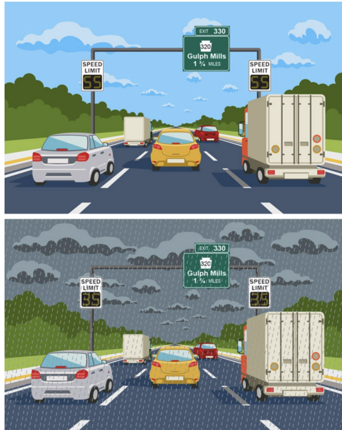
Fig. 4.3: Implementation of variable speed limit. Variable speed limit allows speed limits to be changed based on current road conditions and the level of congestion (original image from PennDOT [1])
