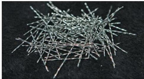
Figure 3.2: Double helix steel fiber (Helix Steel,2013)
