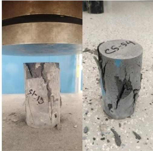
Figure 4.2: Failure mode under compressive strength test
