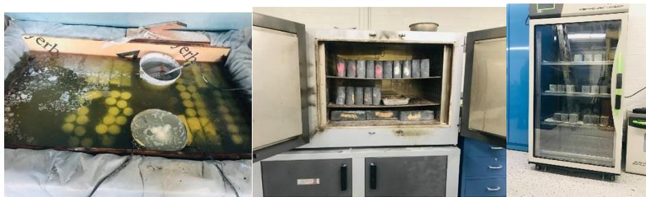
Figure 3.4: Curing in the lime water bath, curing in oven and conditioning in freeze thaw chamber
