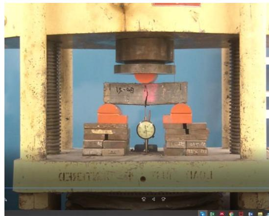
Figure 4.7: Failure pattern of beam specimen under three-point bending test
