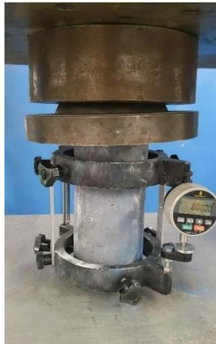
Figure 3.8: Modulus of elasticity test set up
