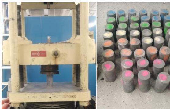
Figure 3.6: Compressive strength test set up and cylinder specimens
