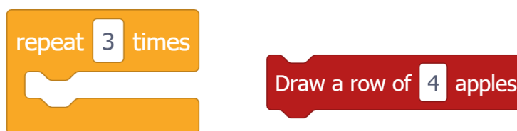
Fig. 3.1: The orange block on the left (Repeat Row) loops over and executes its content the specified number of times. The red block on the right (Repeat Item) draws the item a specified number of times. In this case an apple is drawn four times.
