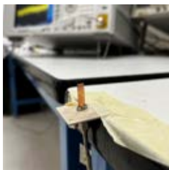
(a) Copper Tape Receiver Antenna
