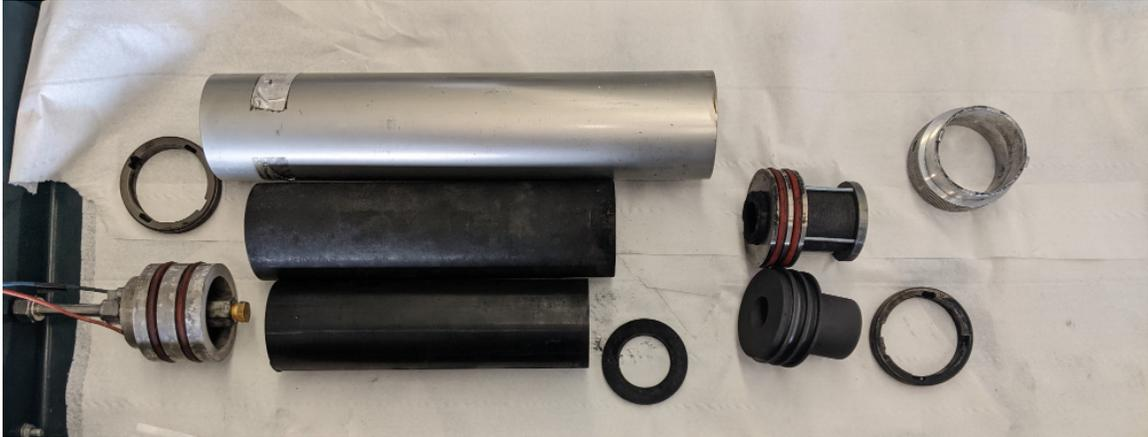
Fig. 3.3: Thrust Chamber Components
