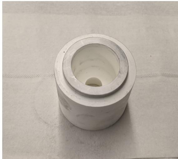
Fig. 2.6: Hexagonal Boron Nitride Insulator
