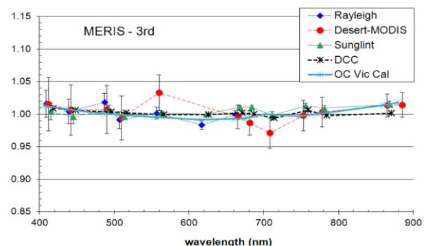
Figure 10. Summary of results obtained through various methods, Rayleigh, desert, sunglint, clouds, in the case of the MERIS 3<sup>rd</sup> reprocessing. Ocean color system vicarious calibration based on in-situ measurements is also provided for comparison.
