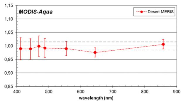
Figure 9. Cross-calibration between MODIS-Aqua and MERIS as a function of wavelength computed over desert sites.
