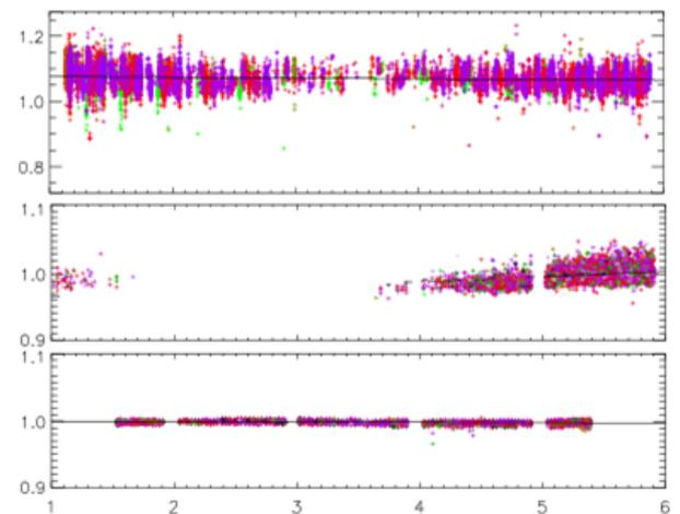
Figure 6. Calibration versus the camera/pixel number for the MERIS band at 620nm, as seen by desert sites (up), Rayleigh scattering (middle), and clouds (bottom).
