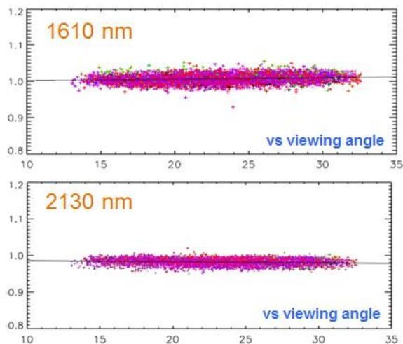
Figure 8. Interband calibration versus the observed reflectance for the MODIS bands at 1610 (up) and 2130nm (bottom) as seen over sunglint assuming the 670nm band as reference.
