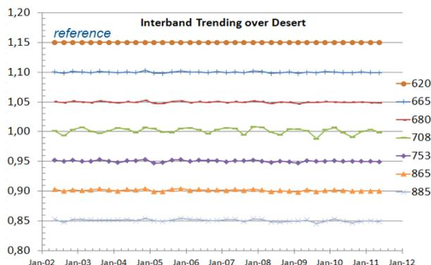
Figure 4. Time series of the inter-band calibration calculated over desert sites for near infrared MERIS bands using the 620nm as the reference band.
