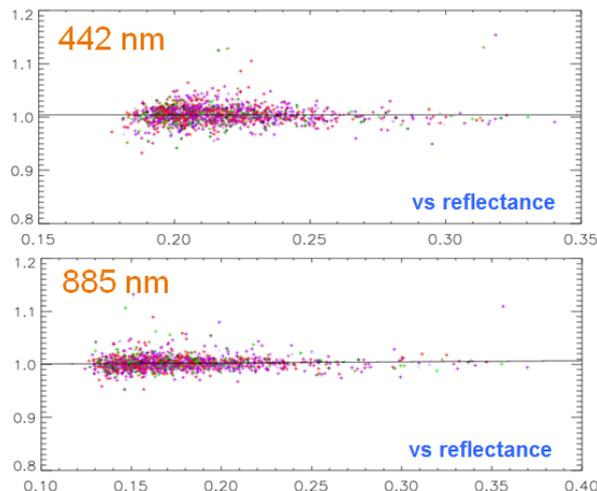
Figure 7. Interband calibration versus the observed reflectance for the MERIS bands at 442 (up) and 885nm (bottom) as seen over sunglint assuming the 620nm band as reference.
