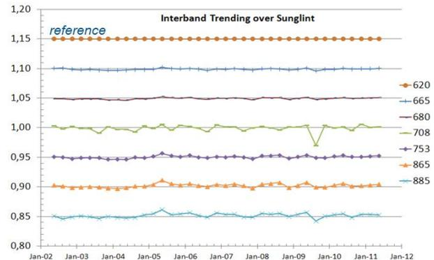
Figure 5. Time series of the inter-band calibration calculated over sunglint for near infrared MERIS bands using the 620nm as the reference band.
