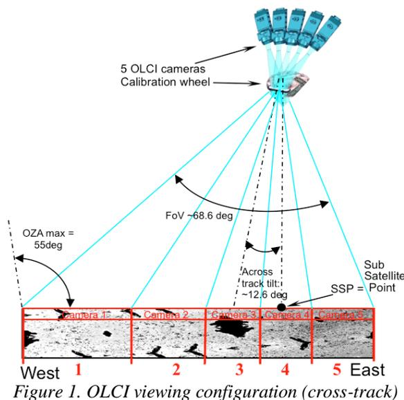
Figure 1. OLCI viewing configuration (cross-track)
