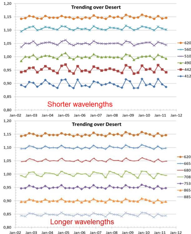
Figure 3. Time series of calibration over desert sites for all MERIS bands. Series are shifted up/down for clarity.
