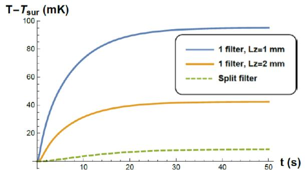
Figure 10b: Transient temperature rise at the center of the back surface for one filter and split filters.
