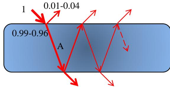
Figure 6. The disposition of radiation by a filter associated with a single incident ray.
