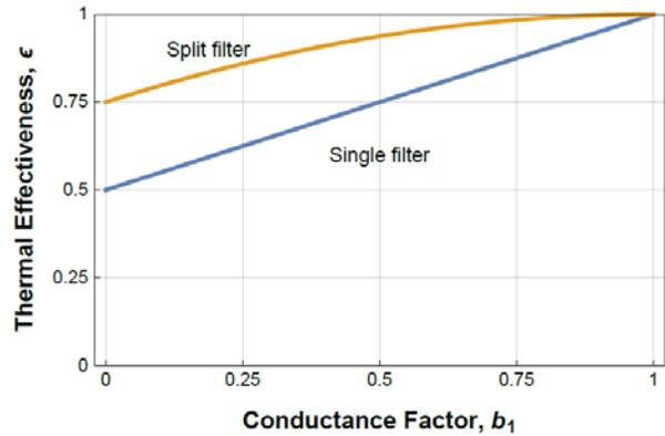
Figure 3. Comparison of thermal effectiveness of the single- and double-segment filters.
