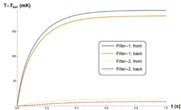
Figure 9b: Transient temperature rise at the center of the surfaces for the split filter.
