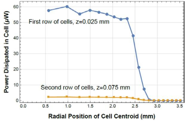
**Figure 8. Distribution of absorbed LW radiation due to Earth-emitted radiation in the fused silica SW filter (Thickness = 1.0 mm, Filter Transmittance = 0.0066).**
