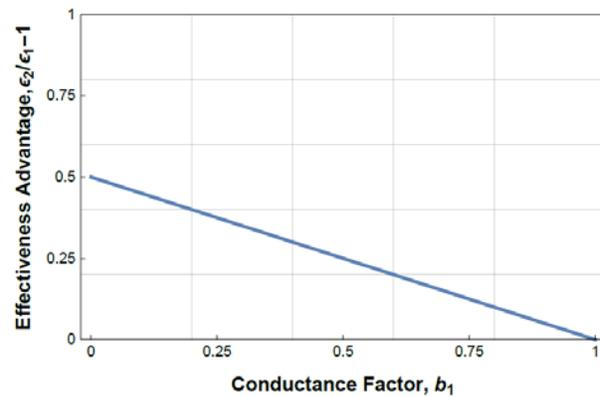
Figure 4. Effectiveness advantage of the double-segment filter over the single-segment filter.
