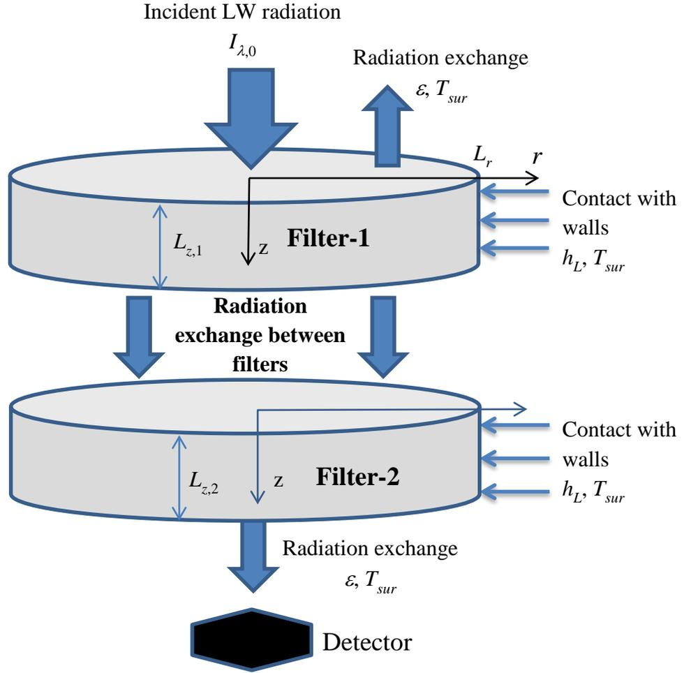
Figure 1: Schematic of the two-filter system.
