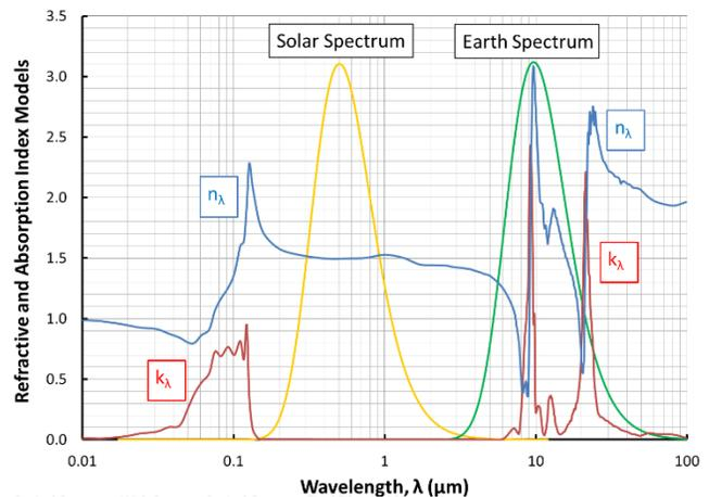
Figure 7. The variation with wavelength of the fused silica optical constants  $n_{\lambda}$  and  $\kappa_{\lambda}$  obtained by averaging the extensive dataset in Kitamura, et al.<sup>3</sup> (solar and Earth-emitted blackbody spectra are superimposed).
