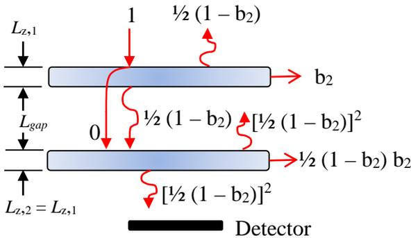
Figure 2. Split-filter model for the special case of  $L_{z,1} = L_{z,2}$ .
