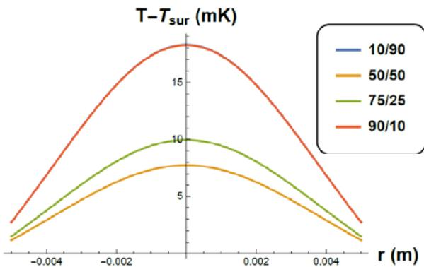
Figure 11a: Steady state temperature rise over the back surface.
