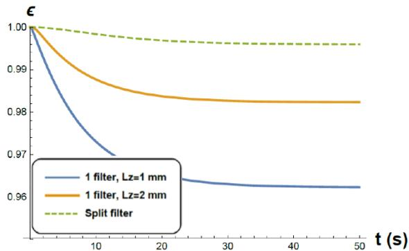
Figure 10c: Thermal effectiveness for one filter and split filters.
