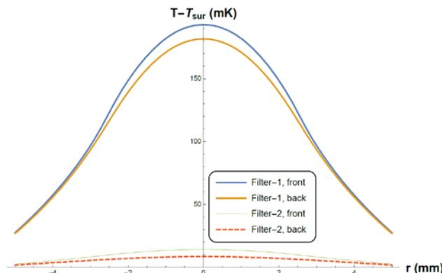
Figure 9a: Steady state temperature rise at the surfaces of the split filter.
