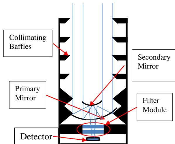
Figure 5. Schematic representation of a typical Earth radiation budget instrument.
