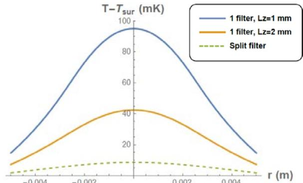
Figure 10a: Steady state temperature rise over the back surface for one filter and split filters ( $L_{z,1} = L_{z,2} = 0.5$  mm).
