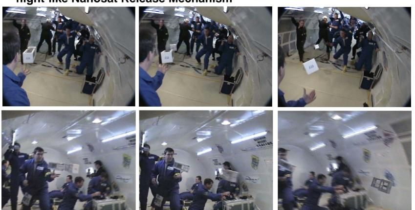
Off-nominal tether deployment tests with fast and slow tumbling deployers performed – all successful
