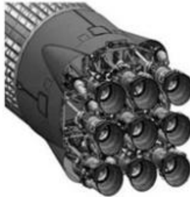
Gimbaled & Variable Thrust Engines of SpaceX's Falcon 9
