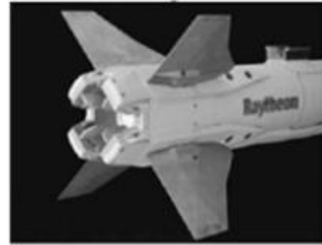
Jet Vanes of an AIM-9X Sidewinder
