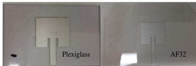
Printed 4.9 GHz solid patch antenna on two different substrates
