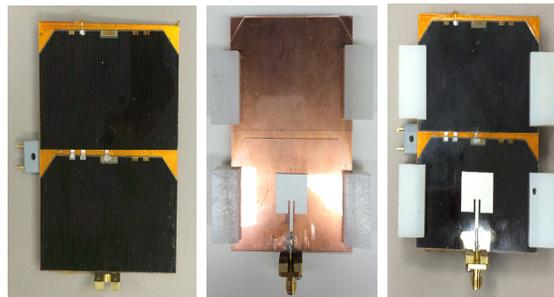
Assembly of antenna with and without solar cells
