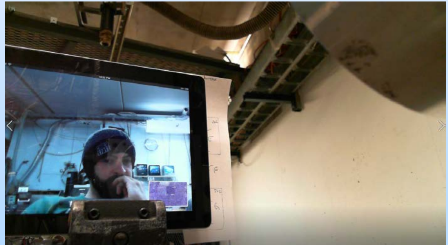
Photo: Irradiation of iPad at UC Davis – due to spot size, multiple irradiation sites were necessary.
