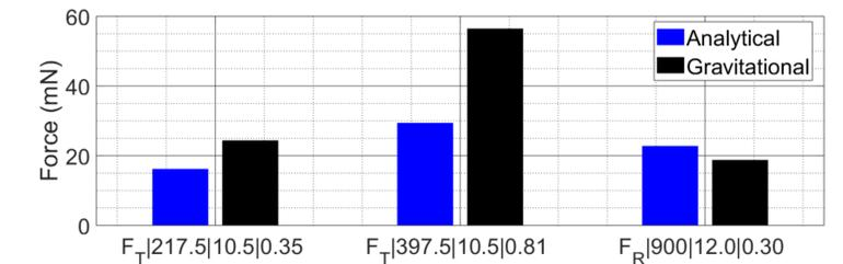
Figure 5. Comparison of the gravitational force due to the incline and the corresponding steady-state force components for each actuator. Labels give the actuator type | angular velocity (rpm) | separation (mm) | incline ( $^{\circ}$ ).
