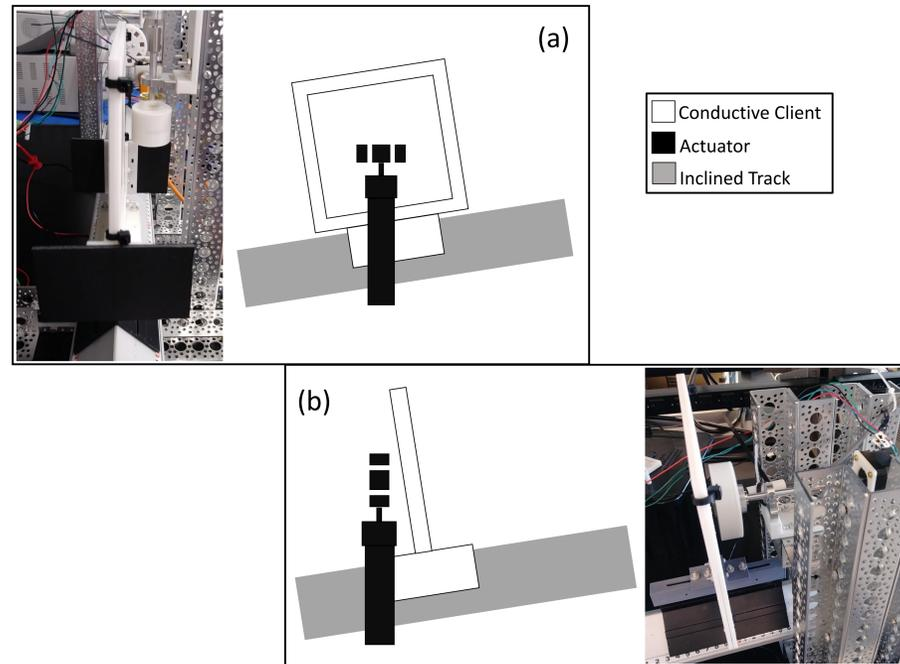
Figure 2. Tangential (a) and normal (b) air track test setups.
