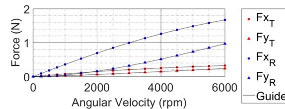
Figure 3. Tangential and normal force components over angular velocity with a separation of one centimeter and negligible relative velocity.
