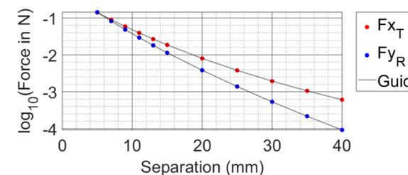
Figure 4. Tangential (600 rpm) and normal (900 rpm) force components over separation with negligible relative velocity.
