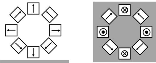
Figure 1. Tangential (left) and normal (right) permanent magnet Halbach arrays.
