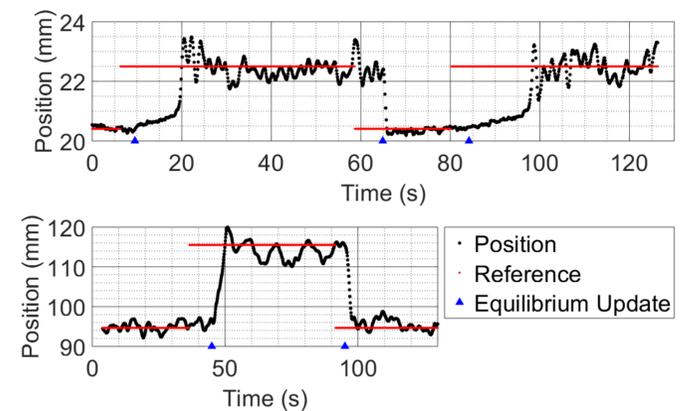
Figure 6. Normal (upper) and tangential (lower) position tracking at a  $0.35^{\circ}$  incline using proportional-derivative control for the linearized systems.
