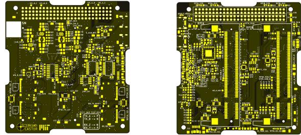
**Figure 6: Beavercube Flight Computer Board Rev 1.0. Key features include 2 onboard Raspberry Pi (RP) compute modules, 4 switching voltage regulators for RP power, embedded micro-USB flash port, 7-port USB hub, 4 micro-SD card slots**
