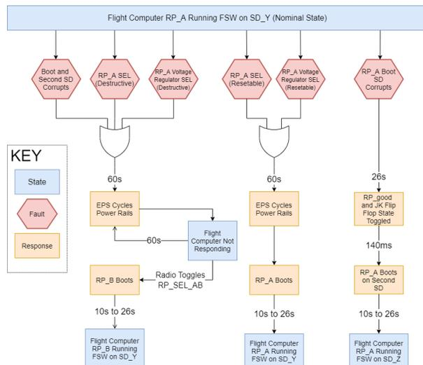
**Figure 4: FDIR system overview.** The transition time between states is indicated. Time to recover from a non-responsive flight computer is dependent on detection by a ground station and subsequent command uplink to toggle RP\_SEL\_AB. Assumes the flight computer powers on with RP\_A booted to SD\_Y
