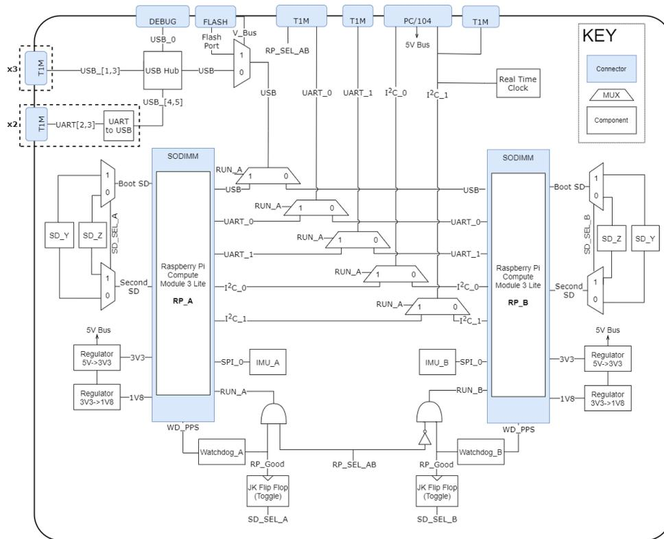
Figure 2: BFC Functionality and Interfaces, Rev 1.0, 4/24/2020
