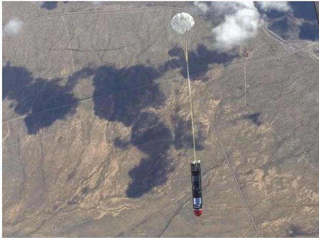
*Figure 8. MIURA 1 parachute system drop test in Eloy, Arizona*
