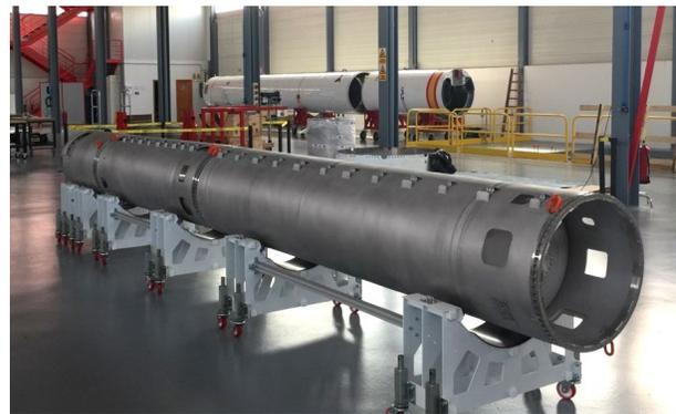
*Figure 11. Stainless steel mock-up of the MIURA 1 tanks (foreground) and MIURA 5 drop test mock-up (background)*
