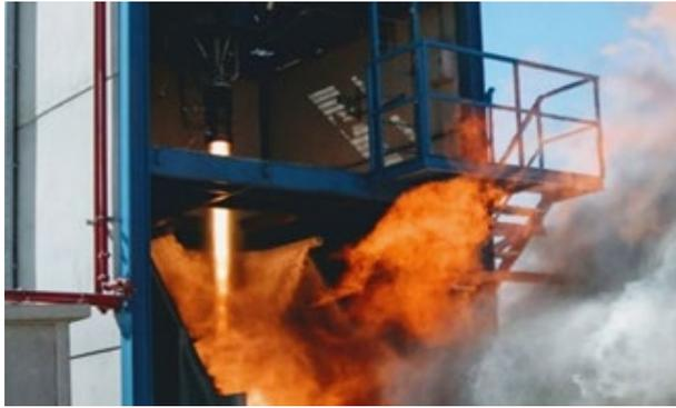
*Figure 1. Test version of the TEPREL engine being fired in the propulsion test facilities of PLD Space*
