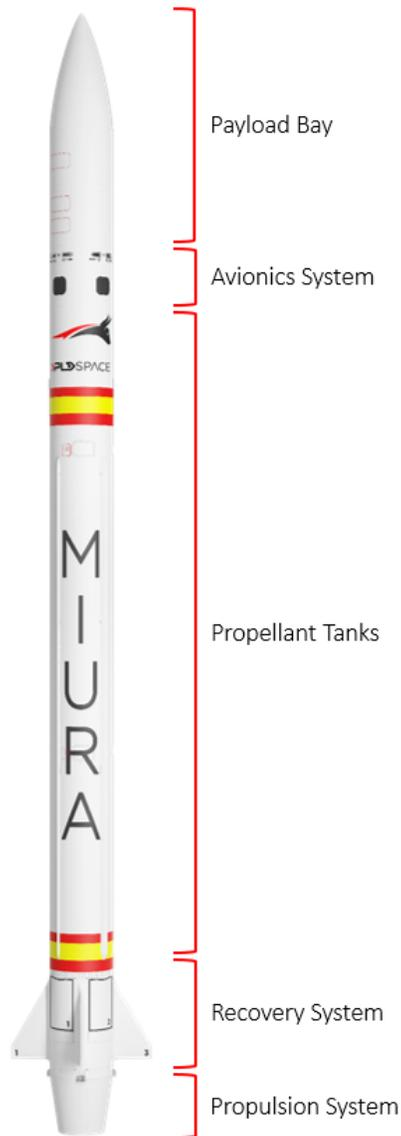
Figure 4. MIURA 1 vehicle subsystems
