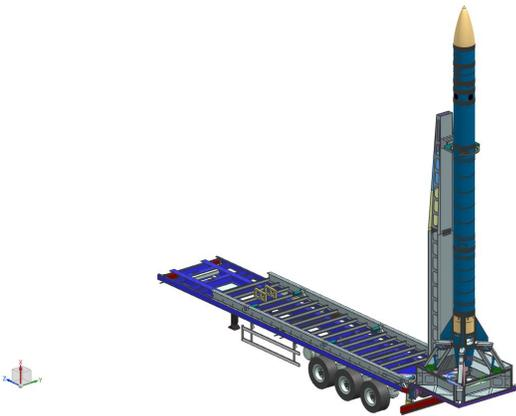
Figure 7. 3D-Model of the mobile launch ramp for MIURA 1 in launch setting
