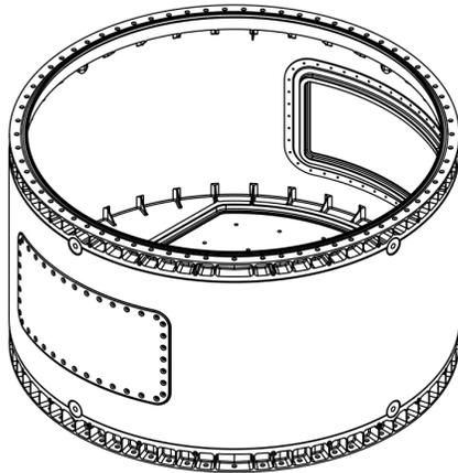
Figure 5. CAD illustration of a Payload Compartment
