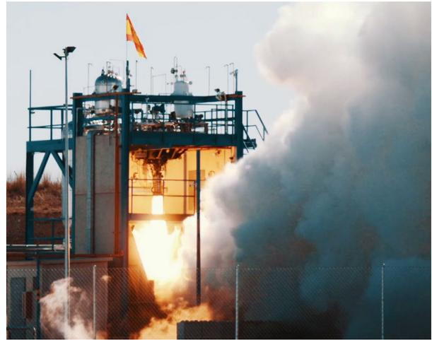
*Figure 10. Flight version of the TEPREL engine being fired in the propulsion test facilities of PLD Space*
