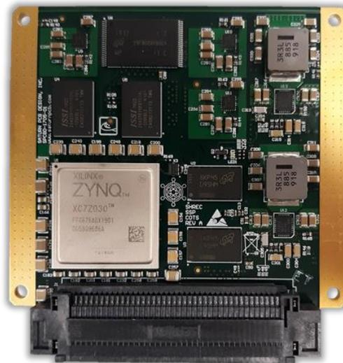
**Figure 4: COTS SSP Rev. A (Engineering Model)**
