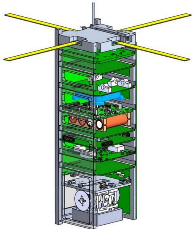
**Figure 3: MiTEE-1 Structural Design Exemplifying Backplane Construction**
