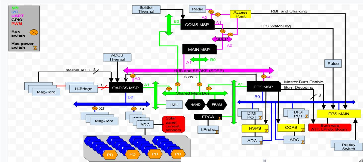
**Figure 2: Computational Architecture Of MiTEE-1**
