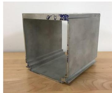
**Figure 4: Waterjet cutting failure with uneven dimensions**
