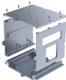
**Figure 3: Exploded view of chassis assembly**
