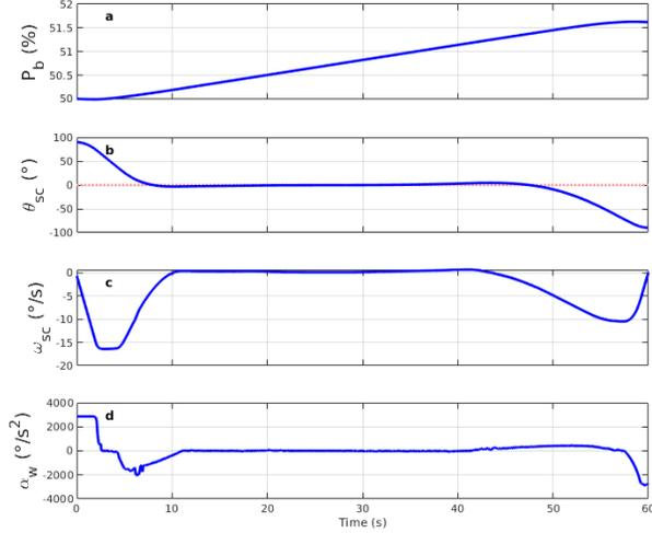
**Figure 6: Satellite system states and input for the “Pass through zero” scenario for slewing between  $90^\circ$  and target at  $-90^\circ$  (b). System states are satellite battery charge (a), satellite angular position  $\theta_{sc}$  (b), and satellite angular velocity  $\omega_{sc}$  (c). Input is reaction wheel acceleration  $\alpha_w$  (d). For panel (b), the dashed red line represents the maximum solar collection angle ( $0^\circ$ ).**
