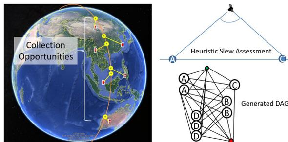
**Figure 1: Representation of a collection planning DAG using target opportunity time discretization and heuristic slew assessment. Opportunities are first calculated (left) and then discretized. A slew heuristic (top right) is then used to determine valid connections between nodes (bottom right).**
