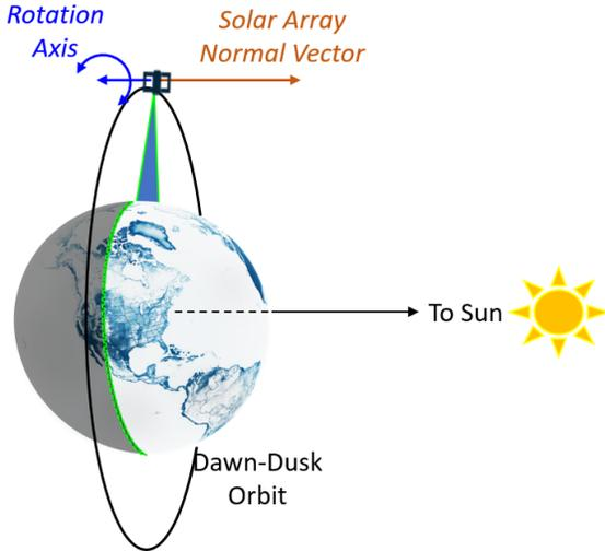
**Figure 4: Illustration of satellite orbit and spacecraft rotation axis relative to orbit position.**
