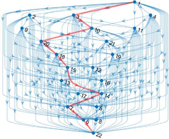
**Figure 2: Example of a collection planning DAG connecting target opportunities. Blue lines represent feasible paths between time-target pairs based the slew time assessments. The optimal collection path is highlighted red.**
