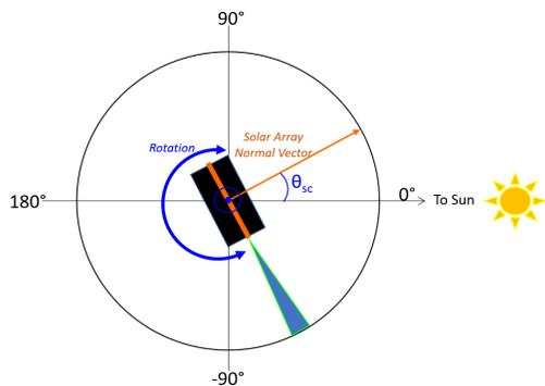
**Figure 5: Spacecraft rotation frame and defined measurement of  $\theta_{sc}$  relative to sun vector.**
