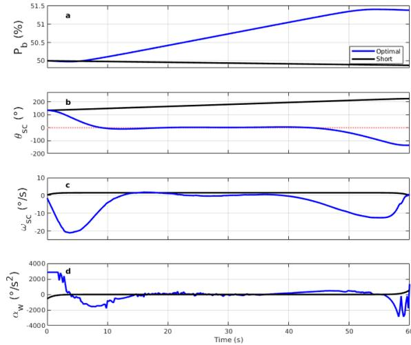
**Figure 7: Comparison of a path for optimal power state (“Optimal”) with a direct path that disregards power collection (“Short”). See Figure 6 for explanation of panels and axes. Slew begins at  $135^\circ$  and terminates at  $225^\circ$  (reference panel b). For panel b, the two trajectory endpoints are equivalent ( $225^\circ = -135^\circ$ ).**
