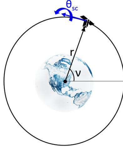
**Figure 3: Illustration of satellite orbital position vector, true anomaly ( $\nu$ ), and the spacecraft angular position ( $\theta_{sc}$ ).**
