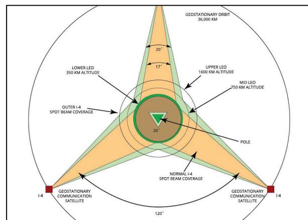
Figure 1 The IDRS System Concept – Polar View
