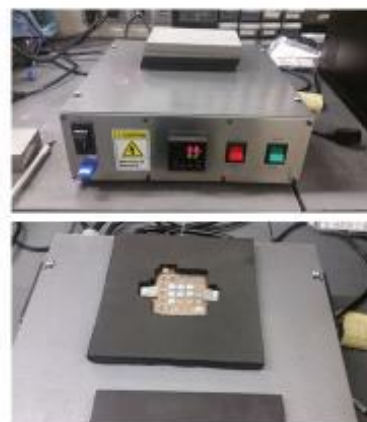
Figure 6. Thermoelectric Test Stand for DSC Sample Cycling
