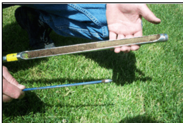
Both soil and tile probes show similar depths of water movement (~ 6 inches in this example).
