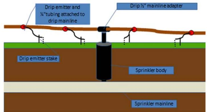
**Figure 5.** Drip conversion adapters such as this one can quickly modify an existing sprinkler body to a 1/2" drip mainline. Following this change, drip emitters and 1/4" drip tubing can be attached to irrigate individual plants.
