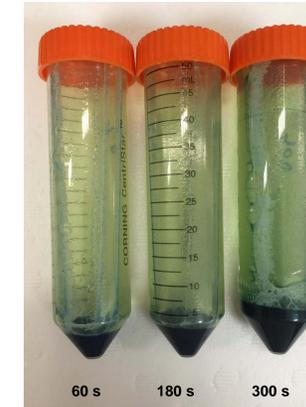
Figure 3) Following centrifugation, at left, the pellet size of longer sonication times increased (revealing a greater phycocyanin yield). The trial runs photographed at left include 60, 180, and 300 seconds of sonication exposure. (Additional experiments could include weighed samples post centrifugation).
