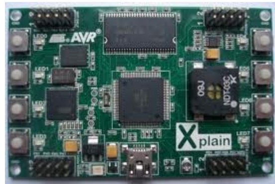
Figure 2: Xplain Hardware Platform
