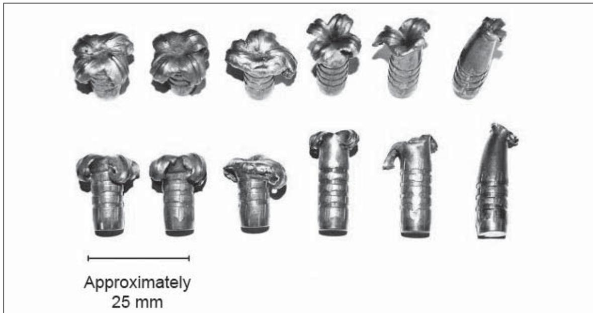
**Figure 3.** A sample of 6 non-lead bullets recovered from elk carcasses at Theodore Roosevelt National Park, viewed from the side (at bottom) and above (at top), demonstrating commonly observed controlled expansion (2 bullets at left) versus less frequent intermediate expansion (center right), occasional fragmentation (center left and second from right), and rare instances of non-expansion and bullet tumbling (at right). (Photo courtesy of Blake McCann)
