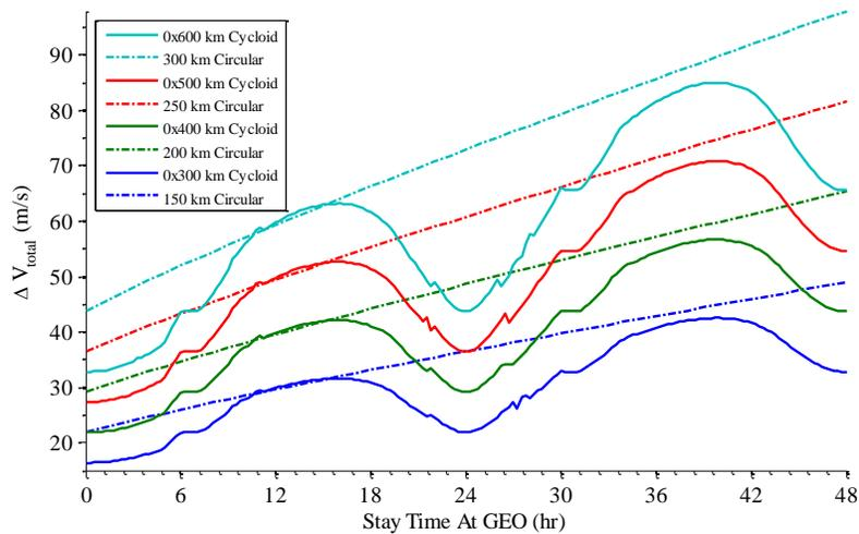
**Figure 3 – Optimal roundtrip in-plane delta-v requirements for a Carrier SmallSat inspection sortie as a function of GEO stay-time/inspection-time. The dash-dot curves show delta-v requirements for different circular Carrier orbits with synodic periods ranging from 3 months to 6 months. The solid curves show delta-v requirements for different cycloid orbits with the same range of synodic periods.**
