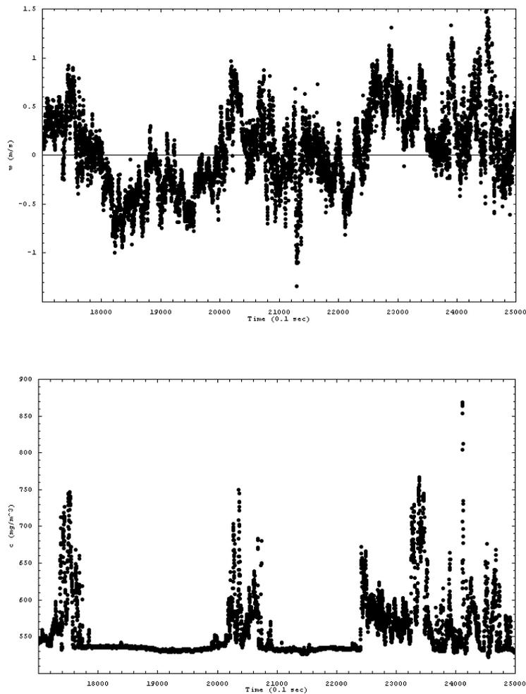
**Figure 2. Time series of vertical velocity and CO<sub>2</sub> density at a height of 12 meters above sources.**
