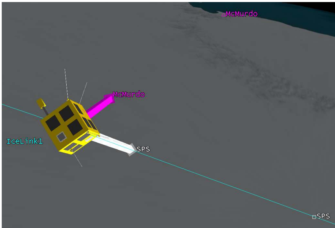
Figure 13. Minimized Approach to Two Target Tracking Using Antarctic Broadband Nanosatellite
