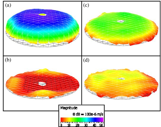
**FIGURE 11. RMS SURFACE VELOCITIES ON THE TRANSMITTING PANEL FOR THREE ACTIVE AND ONE PASSIVE DPAP CONTROL CONFIGURATIONS: (A) PASSIVE, (B) BOTH PANELS ACTIVELY CONTROLLED, (C) INCIDENT PANEL ACTIVELY CONTROLLED, (D) TRANSMITTING PANEL ACTIVELY CONTROLLED (NOTE 0 DB = 100  $\mu\text{m/s}$ ).**
