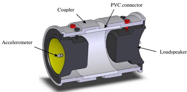
FIGURE 1. CUTAWAY DIAGRAM OF THE DPAP MODULE.
