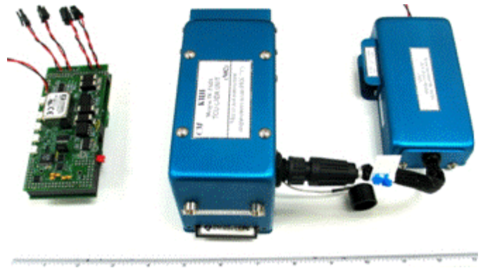
Figure 2. TCU Flight experiment package (center), power module (right), internal electronics (left), and a 12-inch ruler (bottom) for reference
