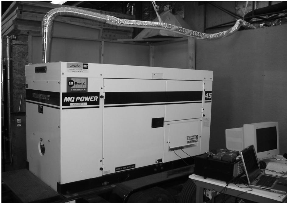
**Figure 1** Apparatus to be controlled: 45KVA (36kW) diesel generator
