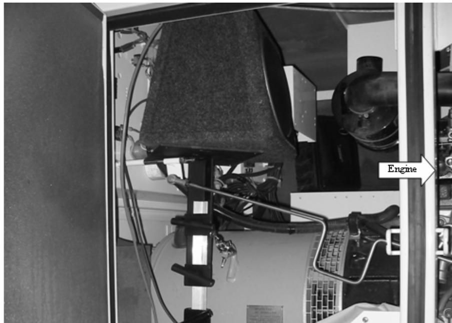
**Figure 3** Control source (8" SUB) mounted inside generator enclosure
