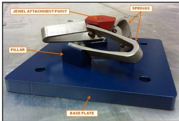
**Figure 13: Photograph of the isolator prototype<sup>12</sup>**
