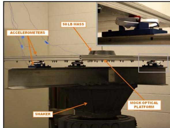
**Figure 14: Mock optics platform and isolator assembly on vibration exciter<sup>12</sup>**
