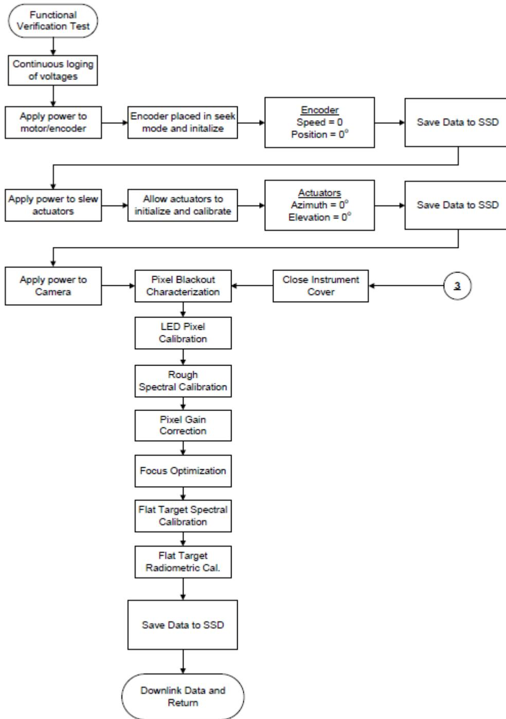
Figure 17: Space-Based CTEEx Functional Verification Test Flow Diagram
