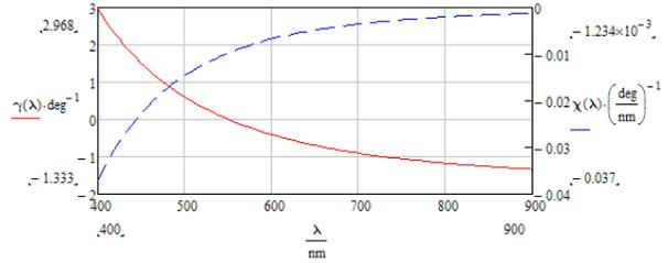
**Figure 3: Theoretical Spectral Dispersion of the CTE<sub>x</sub> Prism<sup>3</sup>**
