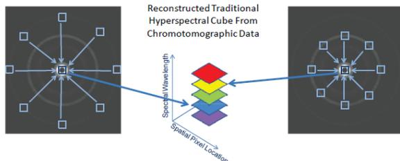
**Figure 5 : Reconstruction of Simulated Chromotomographic Data into a Traditional Hyperspectral Cube**
