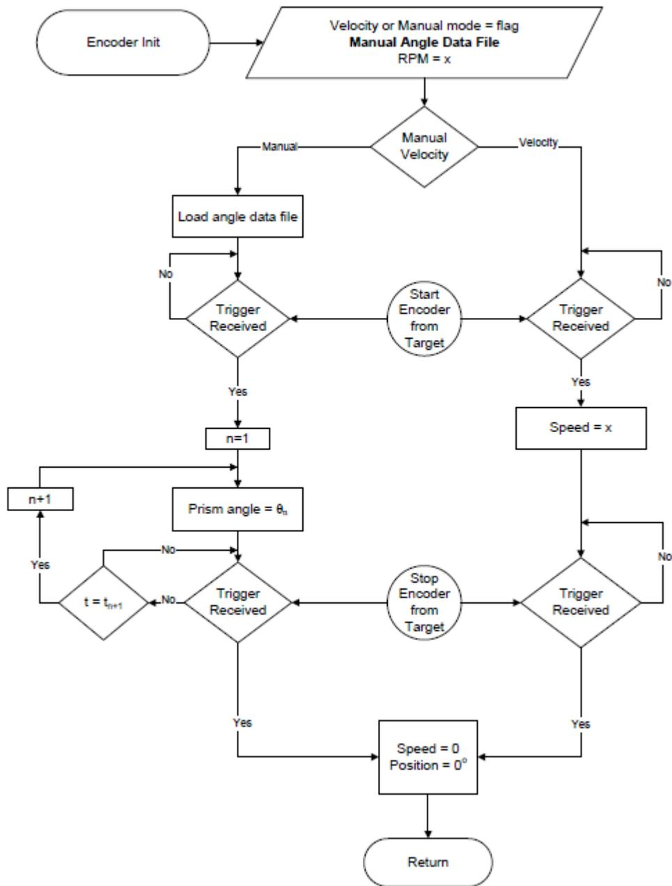
Figure 20: Space-Based CTEEx Prism Control Function Flow Diagram
