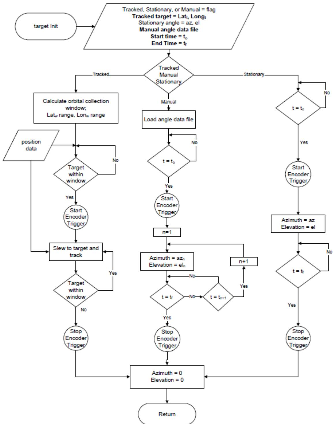
Figure 18: Space-Based CTeX Slewing Control Function Flow Diagram
