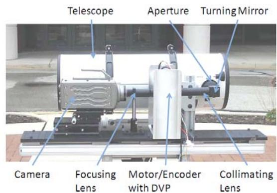
**Figure 7: Completed Ground-Based CTE<sub>x</sub> Instrument<sup>5</sup>**
