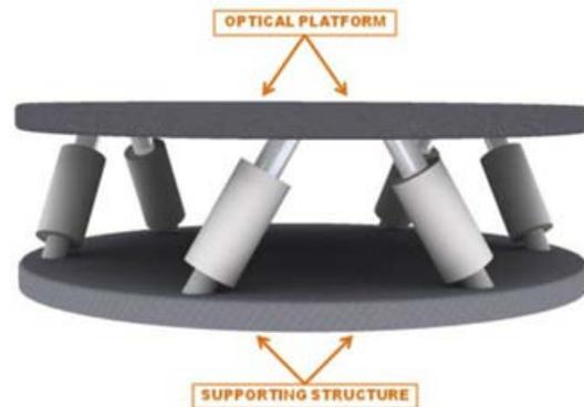
**Figure 12: Hexapod Vibration Isolation Arrangement<sup>12</sup>**
