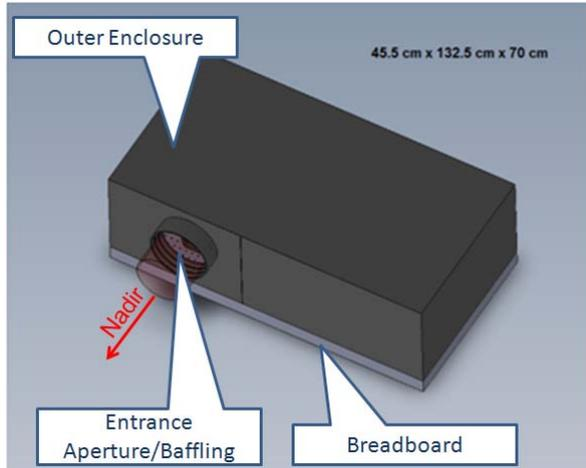
**Figure 9 : CAD Drawing of Off-Axis Mersenne Telescope Enclosure<sup>11</sup>**
