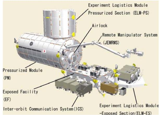
**Figure 8: Japanese E xperimental M odule with Exposed Facility<sup>7</sup>**
