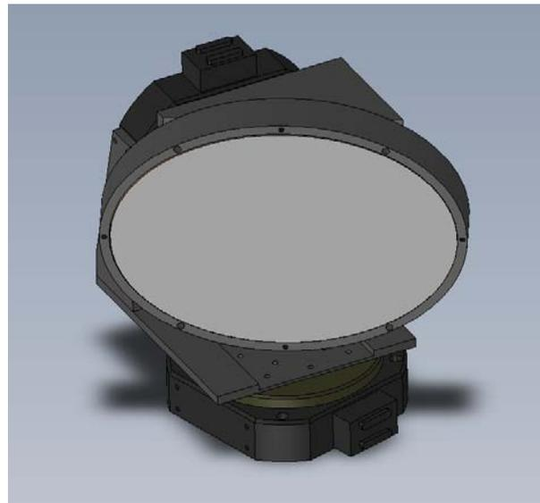
**Figure 11: CAD Drawing of Dwell Mirror Assembly<sup>11</sup>**
