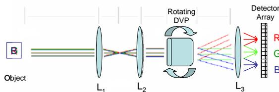
**Figure 6: Schematic of Lab-Based CTE<sub>x</sub> Instrument<sup>1</sup>**
