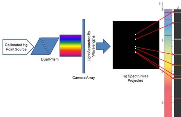
**Figure 2: Spectral Dispersal of an Hg Point Source**
