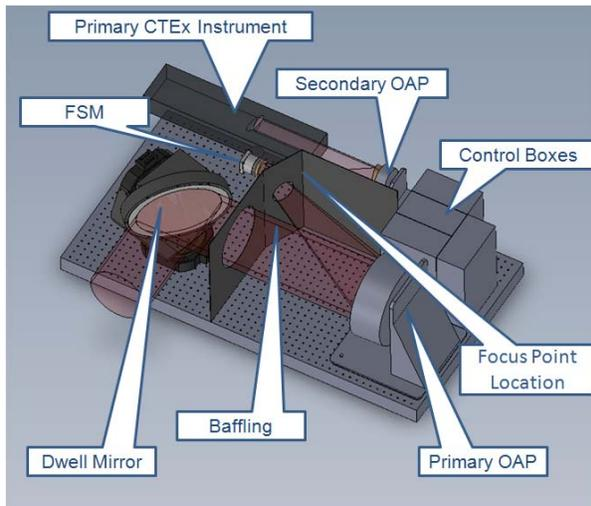
**Figure 10: CAD Drawing of Off-Axis Mersenne Telescope<sup>11</sup>**
