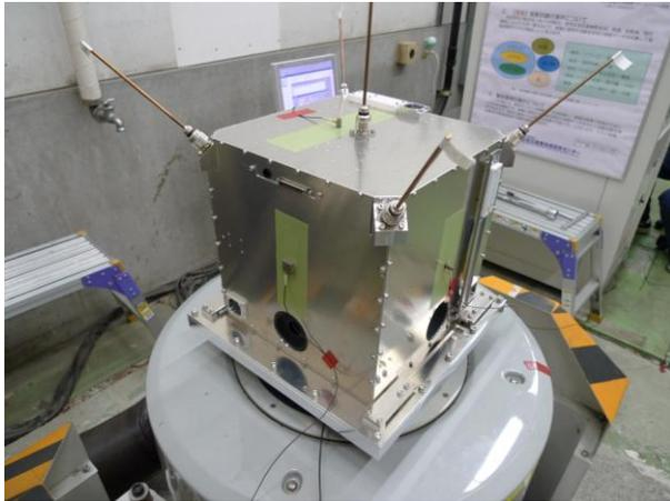
**Figure 21: Vibration test of engineering model**
