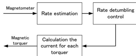
**Figure 18: Schematics of initial attitude acquisition**
