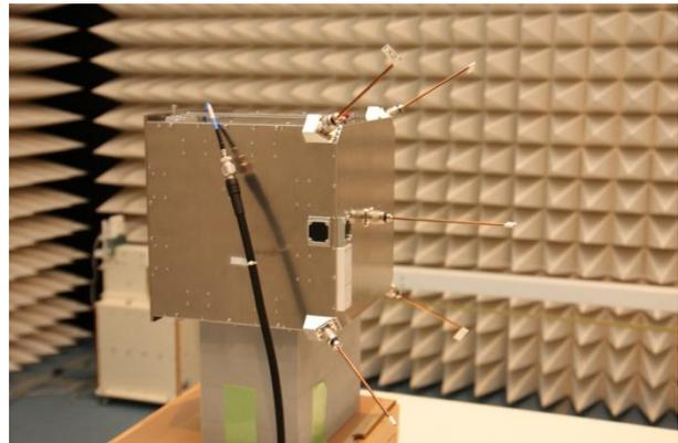
Figure 10: The antenna pattern test
