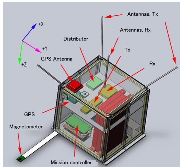
Figure 11: Simplified structure diagram
