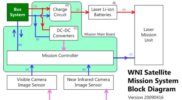
Figure 4: Block diagram of mission system
