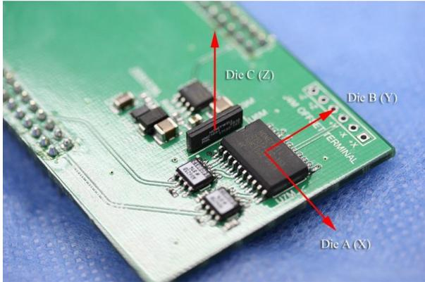
**Figure 13: Magnetometer**
