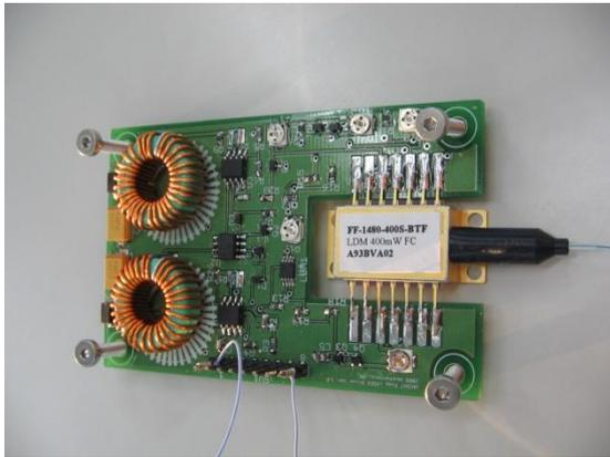
Figure 6: Laser emission unit
