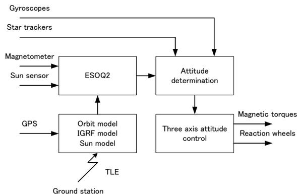
**Figure 19: The three axis attitude control configuration**
