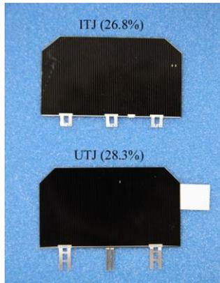
Figure 8: Solar cells
