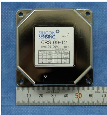
**Figure 14: Gyroscope**
