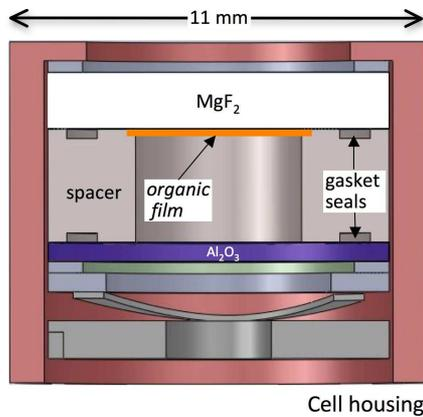
**Figure 8: Reaction Cell Cross Section**
