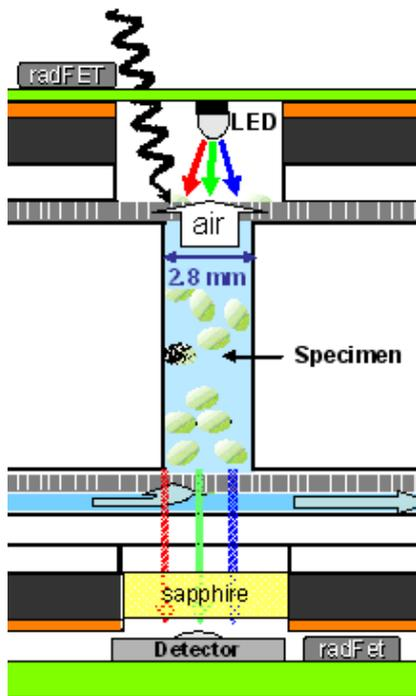
**Figure 6: Sample Well Cross Section**
