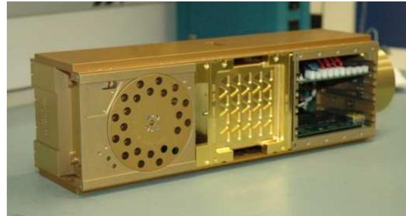
**Figure 2: O/OREOS Prototype Showing Payloads**
