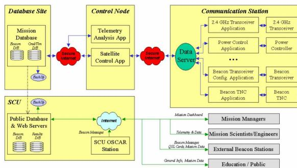
**Figure 13: Distributed Software Architecture**
