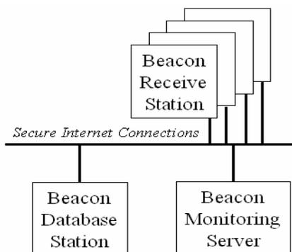
**Figure 16: Beacon Monitoring Architecture**
