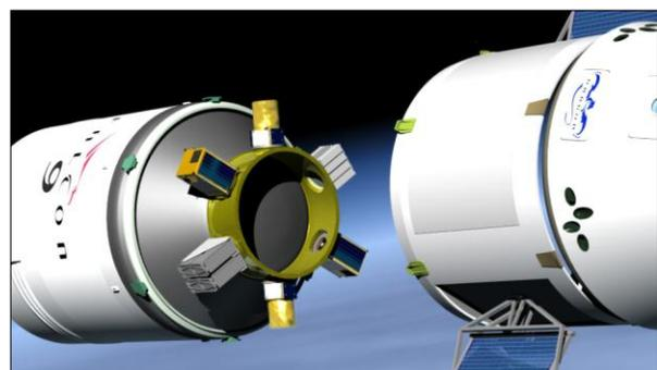
**Figure 3 Falcon 9 Secondary Payload Interfaces**
