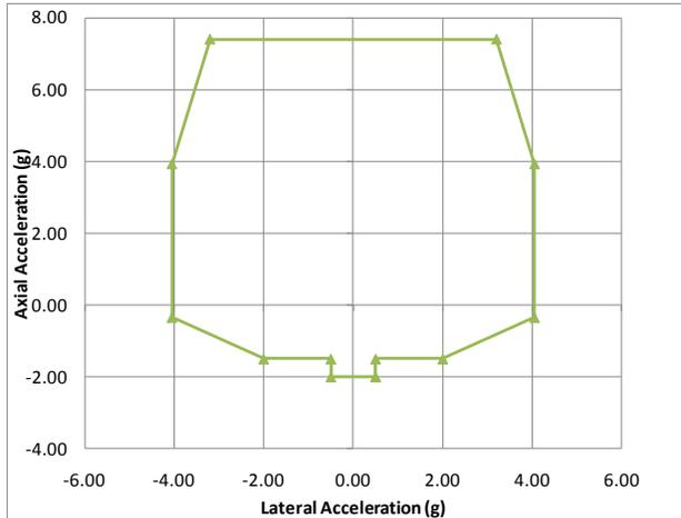
**Figure 12 Launch vehicle Design Load Factors**
