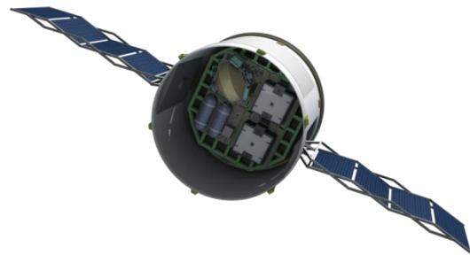
**Figure 10: Cargo Mounted on Cargo Carrier in Dragon Trunk**
