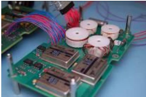
**Figure 5 Engineering Model of the Power Board**
