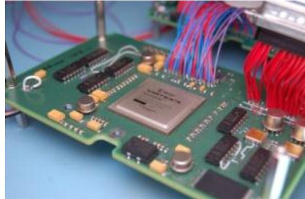
**Figure 6 Engineering Model of the FPGA board**
