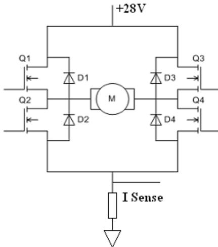
**Figure 10 Example standard single H-Bridge**
