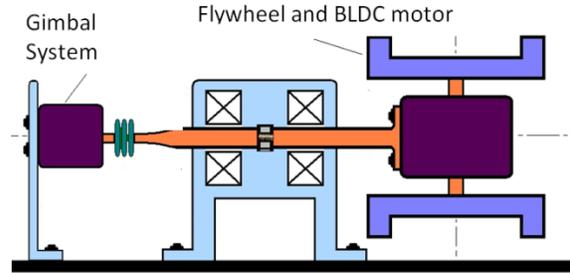
**Figure 2 CMG mechanical configuration**
