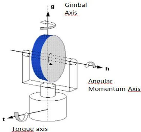
**Figure 1** Conceptual schematic of CMG
