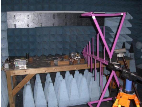
**Figure 12 Radiated Susceptibility testing of the unit**
