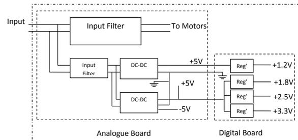
**Figure 7 Block Diagram of the Power Stage**
