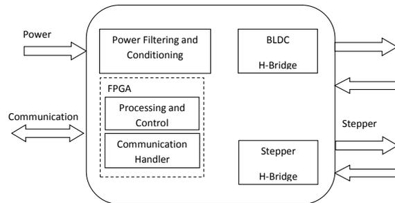
**Figure 3 Top Level Block Diagram of the electronics unit**
