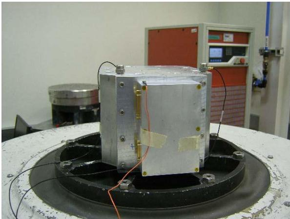
**Figure 13 Qualification model on vibration table.**
