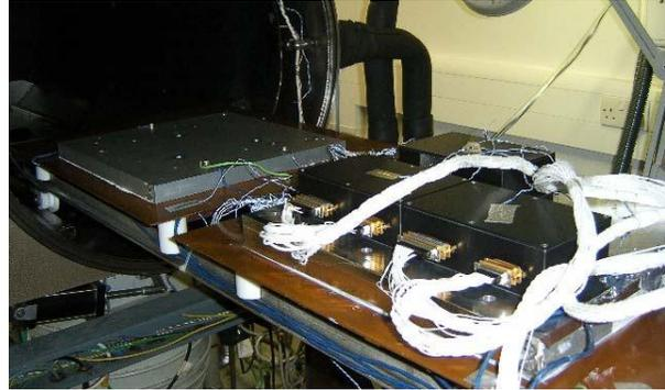
**Figure 14 Flight Models prepared for thermal vacuum testing.**
