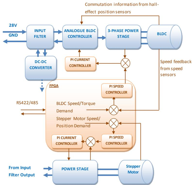
**Figure 9 Block diagram representation of the Motor Control**
