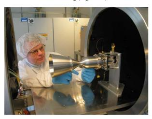
Figure 13: The 220 N HPGP engine (ACE)
