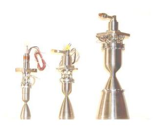
Figure 14: 22 N, 50 N and 220 N HPGP thrusters
