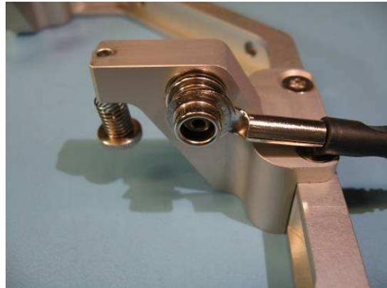
**Figure 4 Snap fastener on MGSE**
