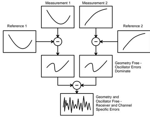
**Figure 5: Measurement Differencing Technique.**
