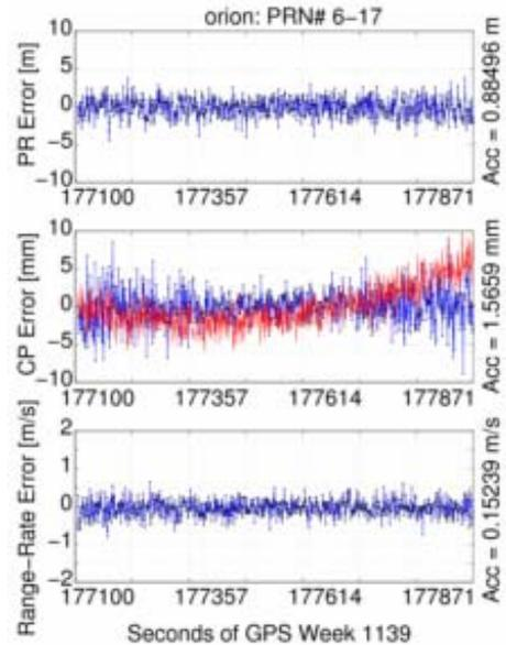
**Figure 7: Orion Systematic Acceleration Dependence Before (red) and After (blue) Tracking Loop Modifications.**
