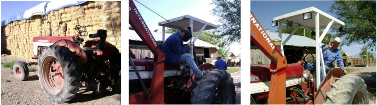
Figure 3. Shade structure added to tractor.
