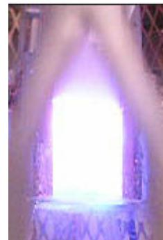
Figure 9. Vacuum test of PPT150 utilizing acrylic housing for visualization.
