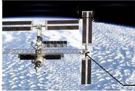
The preferred location for PCSAT2 is out on the ISS Solar array, beyond the alpha joint so that it gets full sun when ISS is in Sun. Our preferred location is shown with the arrow.
