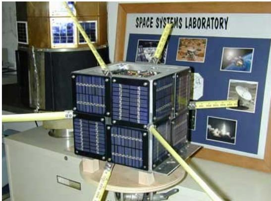
Photo 2. Prototype Communications Satellite (PCsat) with Antennas
