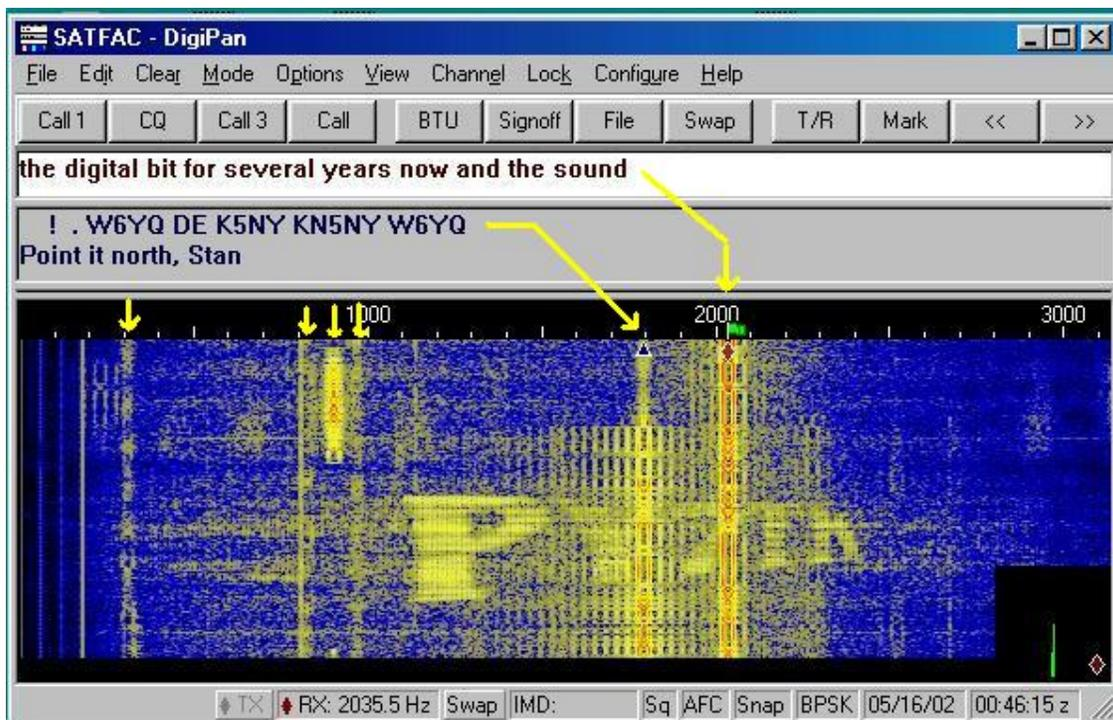
Figure 7. The PSK-31 audio spectrogram showing 7 user signals.
