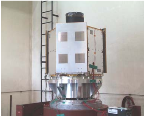
Figure 7. Vibration Test of SM/EOS
