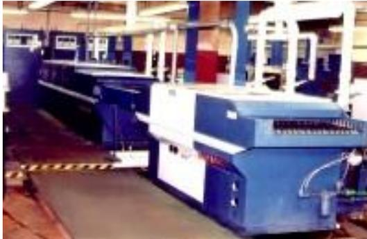
**Figure 4: VACCO Precision Chemical Etching Facility (one of eleven lines)**
